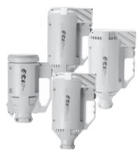
Electric motors are available in 115V or 230V, single phase, 50/60 Hz. All are equipped with 12 ft. (3.5 m) cord, circuit breaker with manual reset, internal cooling fan, and built-in on/off switch. Motors are rated continuous duty.
